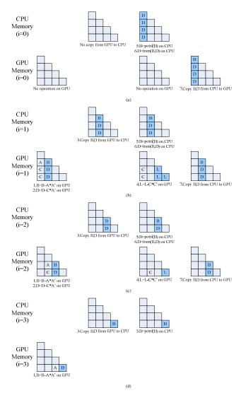
Figure 1. A matrix of 4x4 panels is used to illustrate Volkov's hybrid implementation of blocked Cholesky factorization on CPU and GPU.
