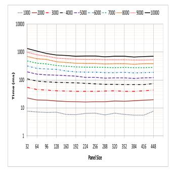
Figure 2. The running time of Volkov's implementation of Cholesky factorization (POTRF) on Fermi GPU for panel sizes 32 to 448 in 32 steps on a matrix of orders 1000 to 10000 in 1000 steps.
