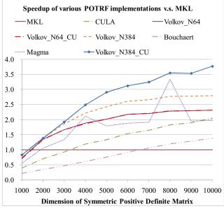
Figure 3. The speedup of various implementations of Choleksy factorization (POTRF) on GPU relative to the state-of-the-art MKL implementation on CPU.
